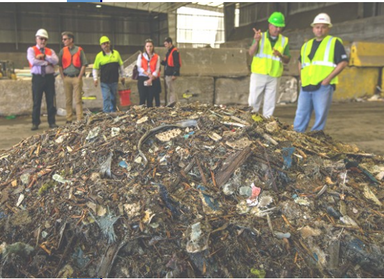
Particles made from deconstructed, ground-up fiberglass boats can be recycled to make concrete for construction projects. (Photo: Ayla Fox)
