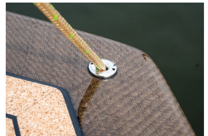
GreenBoats' Flax 27 is a composite of flax fibers and infused resins that are partially bio-based, left. Cork decking, above, also enhances this boat's end-of-life recyclability. The Germany-based company also makes flax components for the IMOCA 60s that are competing in The Ocean Race.
