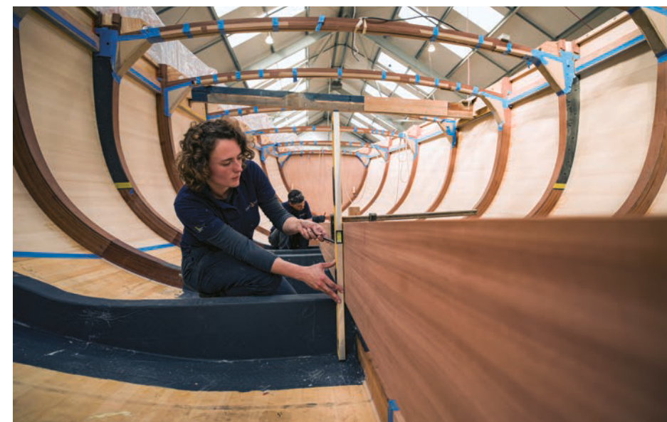
Spirit Yachts uses meticulously sourced woods in their traditional construction techniques, above. The Spirit 30 is coated in an outer skin of flax, rather than traditional fiberglass, using a bio-based resin.
