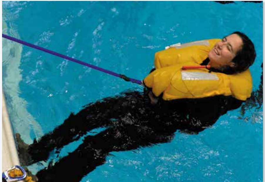
Even with a tethered victim, lifting them aboard presents several challenges. As pool practice sessions revealed, it is possible for the victim to slip out of a loose harness.
