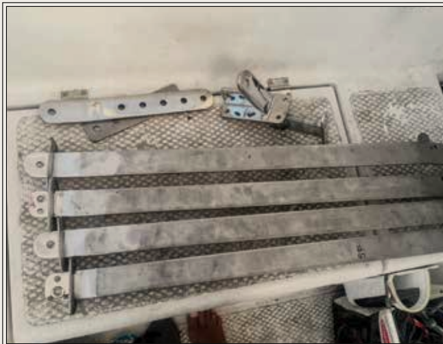
As part of Quiver 's extensive refit, I removed the old chainplates (top left) and replaced them with a new set, and also added a new stem head fitting (left). Another big job was designing and fabricating a hard dodger that also works well as a mount for a pair of flat solar panels (above).
