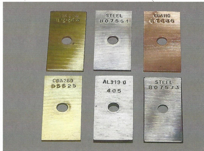
With no anti-corrosion additive present, venting the tank allows in moisture, which leads to corrosion, at left. Sealing the tank to keep moisture out helps prevent corrosion, at right.
