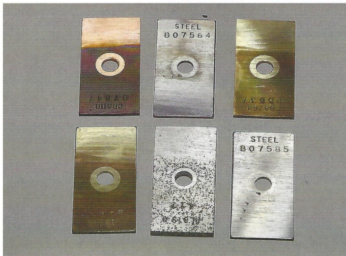
With no anti-corrosion additive present, venting the tank allows in moisture, which leads to corrosion, at left. Sealing the tank to keep moisture out helps prevent corrosion, at right.
