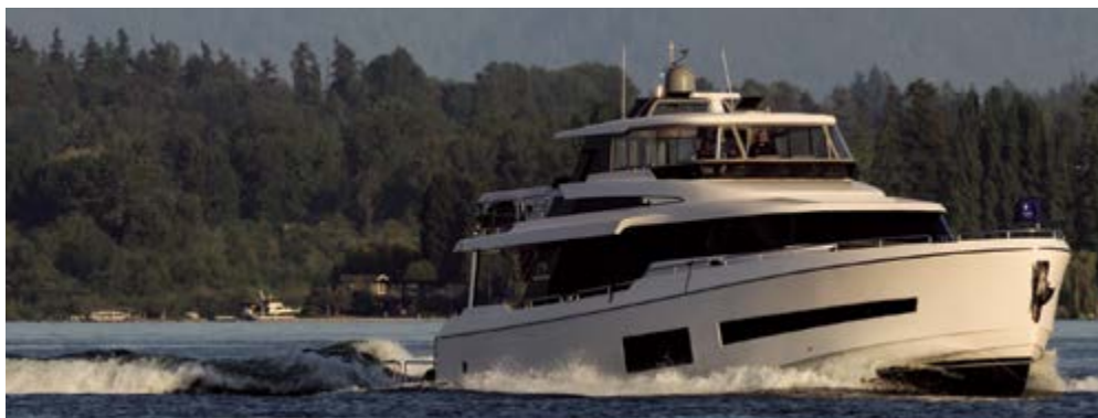
Below: The V68 underway. The twin Caterpillar C18 ACERT engines provide 2,272 horsepower to push this semi-displacement hull to a maximum speed into the mid-20 knot range (photo: Alex Kwanten).
