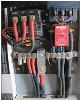
to a source of power other than the battery, and is contained throughout its entire distance in a sheath or enclosure." This exception covers the standard alternator that comes with a marine engine or generator and is wired to the starter motor solenoid, and the batteries, and which is almost never overcurrent protected.
