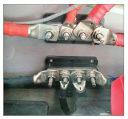
Left and above—Two more examples of unbooted positive bus bars and connections adjacent to negative bus bars in lockers (I see this particularly on catamarans). Although technically ABYC compliant, if there is OCP upstream of the positive bus bars, the installations are all potential fire hazards if loose equipment causes a short circuit.
