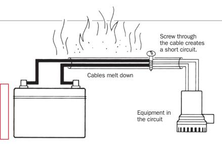
**Above—**When a screw creates a dead short across a circuit, the cables on the positive and negative sides melt down along their entire length, from the source of power (the battery, in this case) to the short. **Top right—**The author created a real-life example of the illustration above: the results of a dead short across a 12-gauge circuit.
