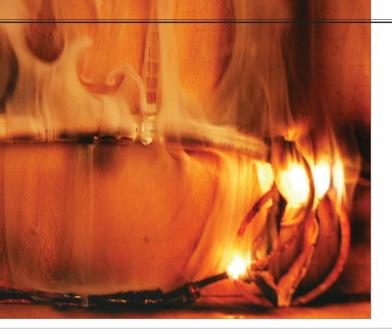
setting the stage for a cable meltdown. All it takes to set things in motion is a short to ground, such as may occur if the insulation is damaged or a terminal comes adrift and contacts a grounded object, or someone installing new cabinetry puts a screw through the wiring.
