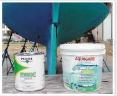
We supplement our panel testing with head-to-head field trials, usually limited to two paints per boat. Our test boats are quartered to ensure equal exposure of both paints..
