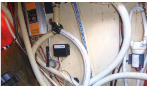
Partway through replacing the hoses and valves; the new intake pump is on the right
