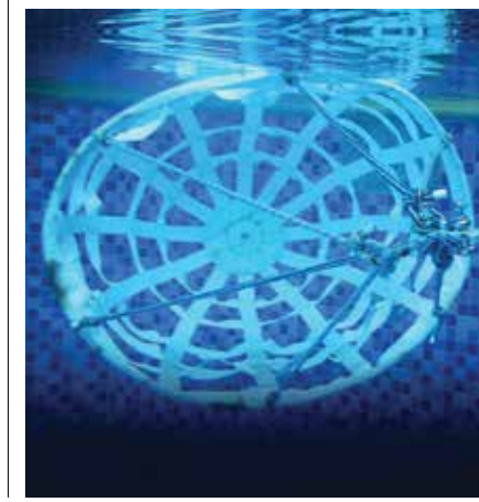
In a swimming pool, the [redacted] deployed a slowing drogue that Carolyn sewed using polypropylene webbing to see how it would set at sea.
