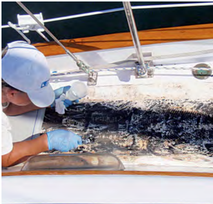
A tedious part of the project was filling the old screw holes with epoxy, above. [redacted] and [redacted] did this before power sanding the deck in preparation for the application of a layer of fiberglass cloth in epoxy resin, near right. After the epoxy had cured in the sun for a week, they sanded it fair, far right, before applying the non-skid finish.
