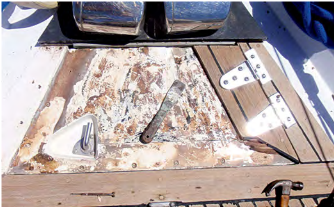
The anchor locker hatch offered an opportunity to test the feasibility of removing the teak decking, above left. The fiberglass deck under the teak was sound enough to stand alone, above right. [redacted] first step in the main project was to cut around the screws, below.
