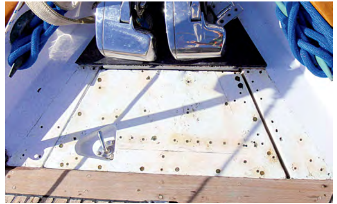
The anchor locker hatch offered an opportunity to test the feasibility of removing the teak decking, above left. The fiberglass deck under the teak was sound enough to stand alone, above right. [redacted] first step in the main project was to cut around the screws, below.
