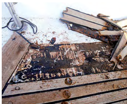
The farthest outboard teak planks were set in a white bedding compound and came up quite easily, at left. As [redacted] worked his way inboard, he found a tar-like compound that was much stickier, center. The teak from then on broke off in smaller pieces, at right.
