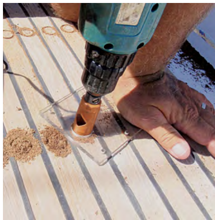
The anchor locker hatch offered an opportunity to test the feasibility of removing the teak decking, above left. The fiberglass deck under the teak was sound enough to stand alone, above right. [redacted] first step in the main project was to cut around the screws, below.
