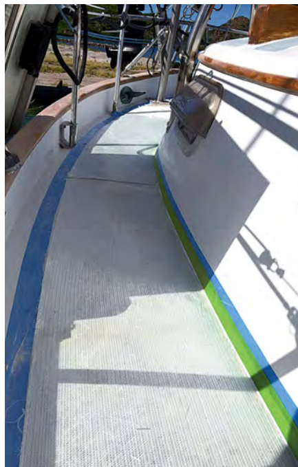
A tedious part of the project was filling the old screw holes with epoxy, above. [redacted] and [redacted] did this before power sanding the deck in preparation for the application of a layer of fiberglass cloth in epoxy resin, near right. After the epoxy had cured in the sun for a week, they sanded it fair, far right, before applying the non-skid finish.
