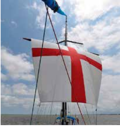
When the wind is astern, a square sail is still a very efficient way to propel a vessel, even today
