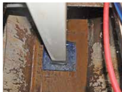
...onto its new stainless steel mast step, which was bolted to the keelson
