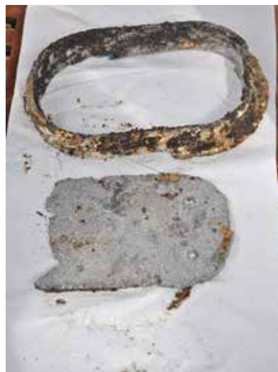
The mainmast step was so corroded it actually split when the mast was pulled out of the bottom of the boat
