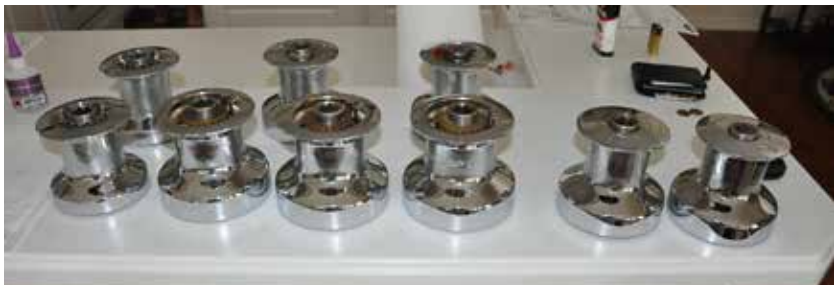
The winches were also re-chromed while they were off the masts
