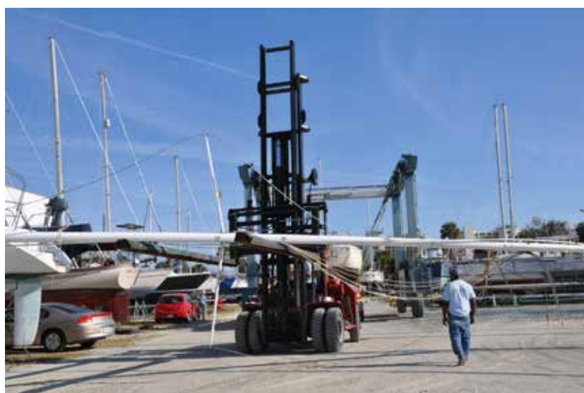
The forklift truck carried the masts to trestles already set up in the boatyard
