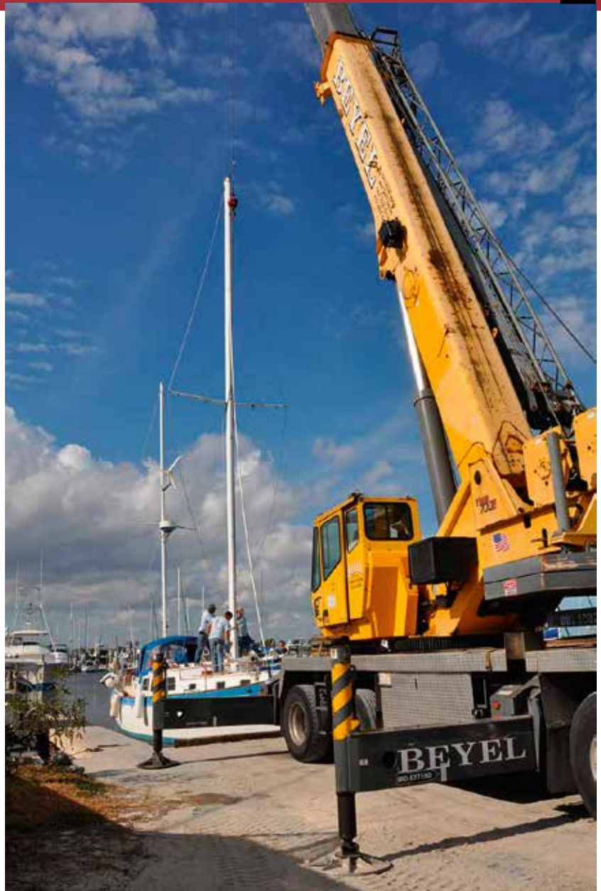
The crane couldn't lift the mainmast and break the joint between the mast and mast step...
