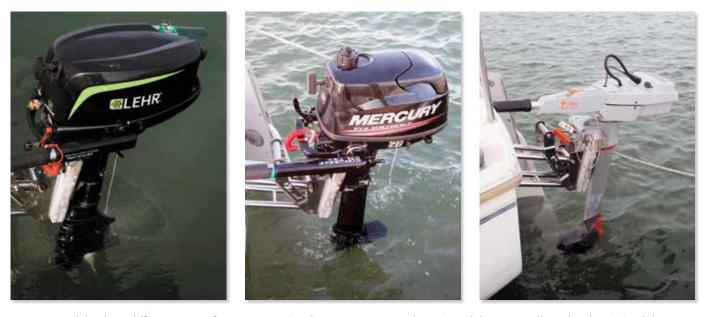
We mounted the three different types of engines on a Catalina 22 to compare them. Speed data was collected with a GPS while steering reciprocal courses at slack tide. From left: 5-horsepower Lehr, 5-horsepower Mercury SailPower, and the Torqeedo Travel 1003.
