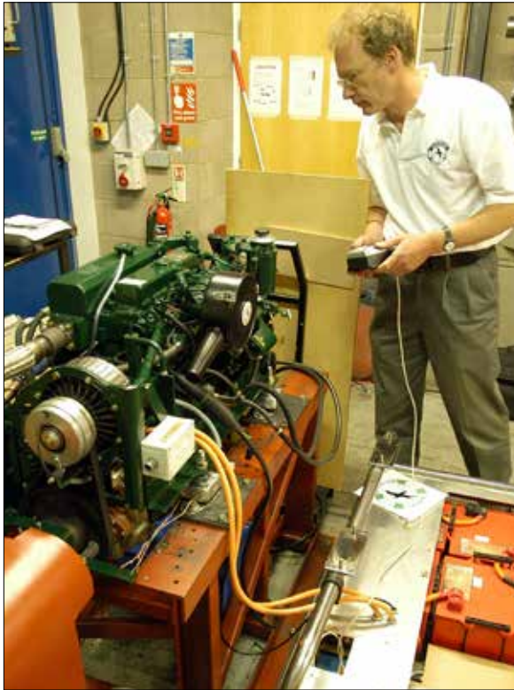
Left —Graeme Hawksley, the founder and owner of Hybrid Marine, testing one of his systems in the Beta Marine factory in the U.K. Above —This detailed system data display and diagnostic tool from Hybrid Marine is representative of those being created by all the hybrid developers. It monitors a lot more than the rpm, temperature, oil pressure, and voltage of a conventional system.
