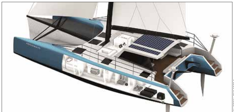
Electric outboard manufacturer Torqeedo is developing a serial hybrid system built around an energy-control module that can be applied to standardized inputs from electric machines, generators, solar, and other sources. This schematic is for a serial hybrid catamaran.
