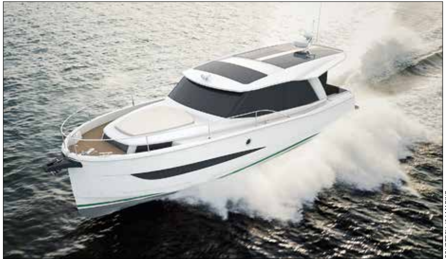
The Greenline 36 (10.9m), the latest in the Greenline family of parallel hybrid cruisers, relies on an integrated flywheel electric machine built into a Volvo Penta D3, and a simple manual selector for electric or diesel propulsion.
