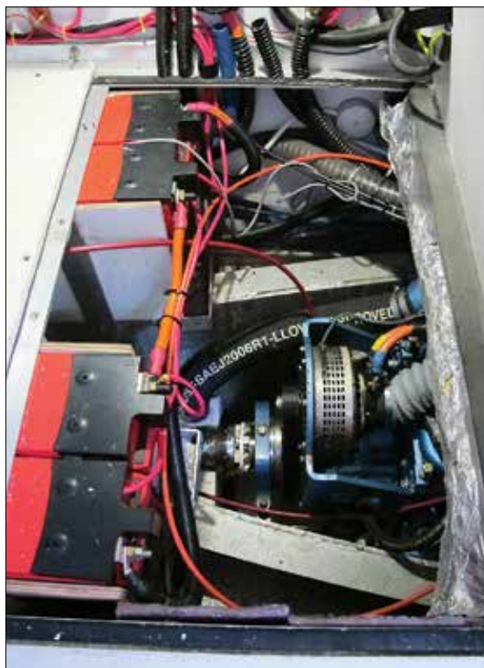
Above —One great benefit of a parallel system to a cruising sailboat is the ability to generate power through a freewheeling prop while under sail. Data for the Hybrid Marine system were collected aboard Seaweed using three different propellers—folding, fixed, and the Bruntons Autoprop.
