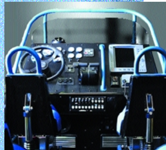
■ Built to withstand radical missions, this 23 1/2-footer is up to any civilian challenge. The aluminum console is rugged and filled with high-tech, military-grade electronics.
