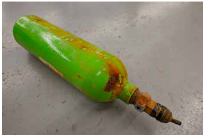
Above: Water trapped inside a vacuum bag past a raft's service date corroded this inflation cylinder and mechanism, leading to a costly replacement. Below: ACR's mobile app provides an intuitive display of test data by connecting to beacons with the same passive Near Field Communication technology that is incorporated into credit card chips.
