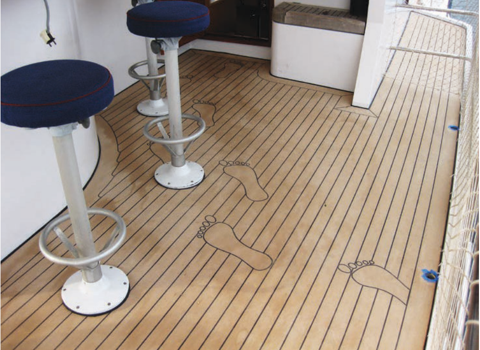
Esthec decking is a composite, and it comes in many different aesthetics to suit different boats. It is made of 25% recycled materials.
