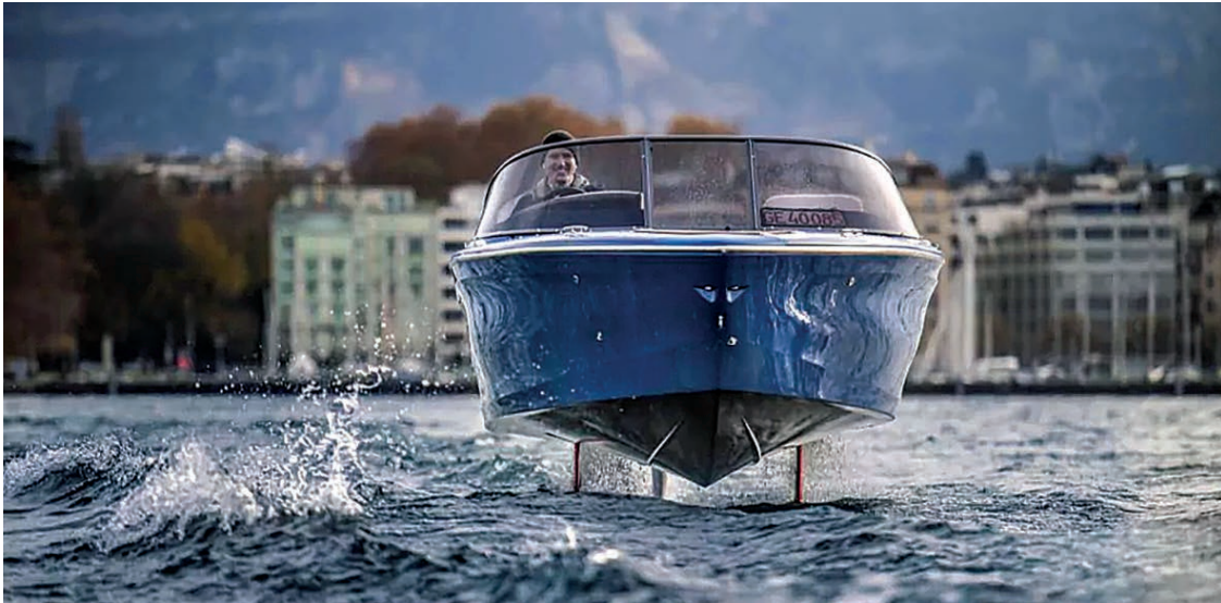
This Candela hydrofoil lifts the powerboat out of the water at speed, thereby substantially reducing drag and slashing fuel use. Candela, known for innovative hull designs, was founded in 2014 with the goal of creating electric-propelled boats with the range of those with internal combustion engines. It has a new investor: Groupe Beneteau, the world’s second-largest builder of recreational boats.
