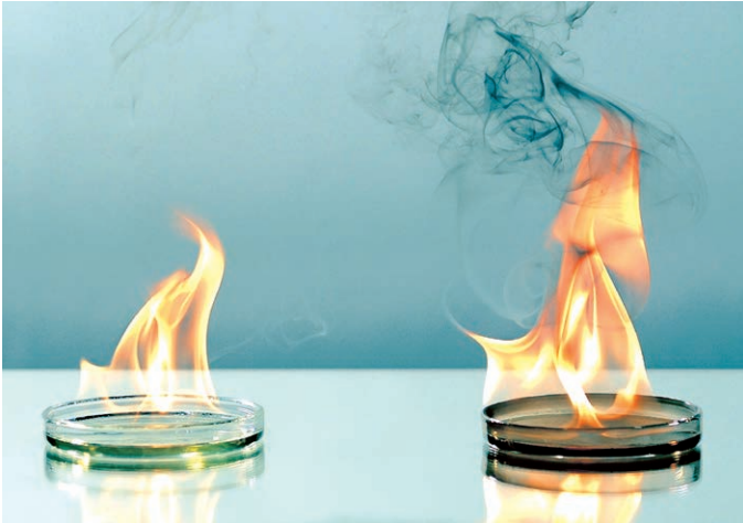
Neste claims its MY Renewable Diesel made from cooking oil, animal fat, and food industry waste (left) reduces CO 2 emissions by 75% compared to conventional fossil-based diesel fuel (right).
