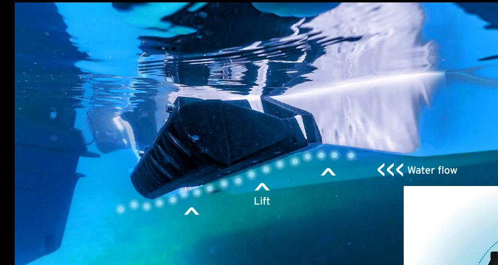
**SEAKEEPR** Seakeeper Ride controllers are mounted to the transom but differ from typical interceptors. Instead of flat blades, Ride’s curved rotary blades (right) make up to 100 adjustments every second to reduce roll, pitch, and yaw. Proprietary hardware and software senses and predicts motion, then automatically responds instantaneously to suppress it before it’s felt.
