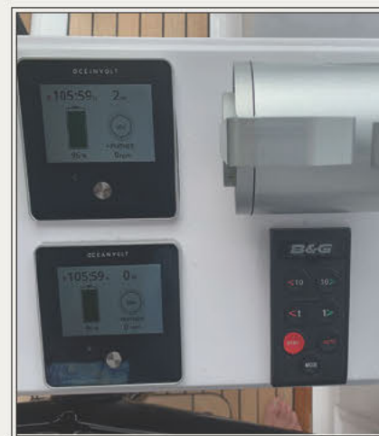
This fall, Green Marine introduced a new all-electric yacht to American sailors: the Salona 46 with two Oceanvolt ServoProps, and the ability to hydrogenerate twice as fast. The Salona features twin control panels and throttles (left), a pair of dedicated Oceanvolt motor controllers (center), and a Victron Energy Quattro charger/inverter (right).
