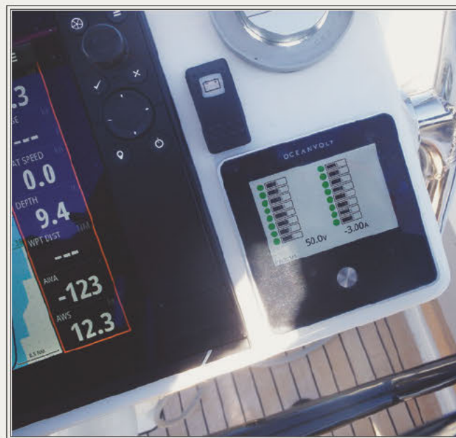
On the Arcona 435Z, the space where you’d normally expect to find a diesel auxiliary is occupied by a bank of lithium-ion batteries (left). Lithium batteries have far greater power density than lead-acid batteries, meaning they’re lighter for a given capacity. The Oceanvolt system allows you to monitor batteries at both the module level and cell level (right).
