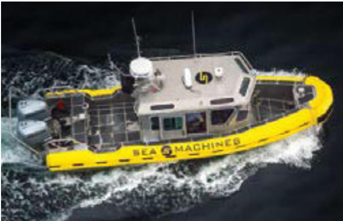
Above: AI-guided boats can be trained to recognize other vessels and objects under real-life circumstances. Below: A SAFE Boat with Sea Machine's autonomous technology. Thanks to numerous sensors already in place, modern recreational boats are good candidates for autonomy.
