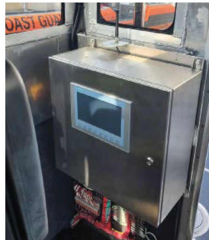
One of several components in Sea Machines' "Intelligence System" that gives a U.S. Coast Guard Defiant 29 autonomous capability.
