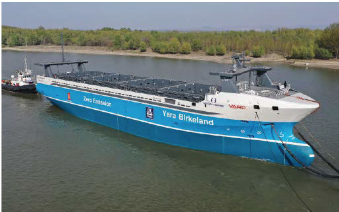
This Norwegian container ship, launched last year, is the first of its kind. Fully autonomous and fully electric, she produces zero emissions.
