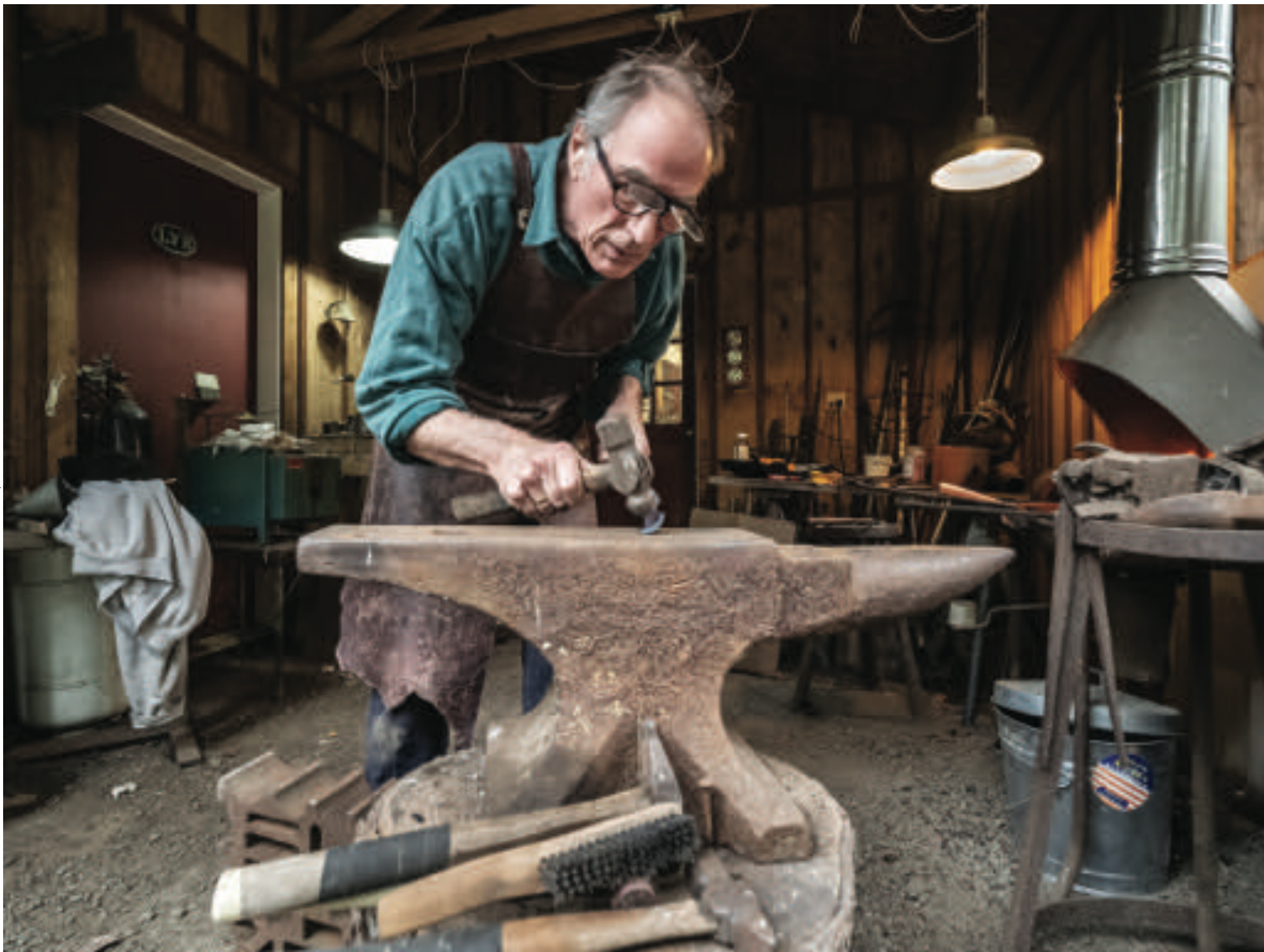
Left: Louchard hammers out a curved gouge from the forge.
