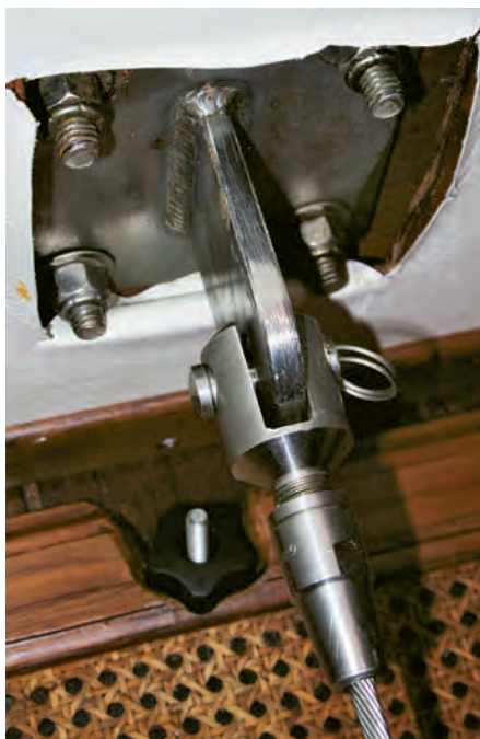
Below, [REDACTED] added a robust deck plate under the foredeck with an eye to accept a turnbuckle and wire (at left) that transfers the load to the foremost interior bulkhead, which is glassed to the hull. (at right).
