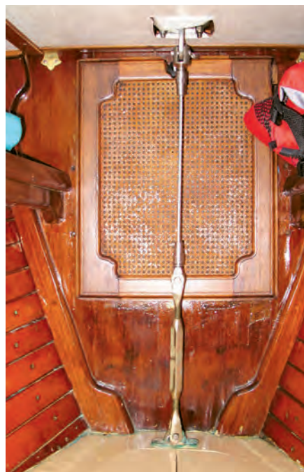
Below, [REDACTED] added a robust deck plate under the foredeck with an eye to accept a turnbuckle and wire (at left) that transfers the load to the foremost interior bulkhead, which is glassed to the hull. (at right).
