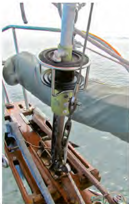
In the forward position, the stay is attached to a permanent toggle installed in the stemhead fitting's aft-most opening. The stay is just clear of the furling drum and allows for easy hoisting and lowering of sails.
