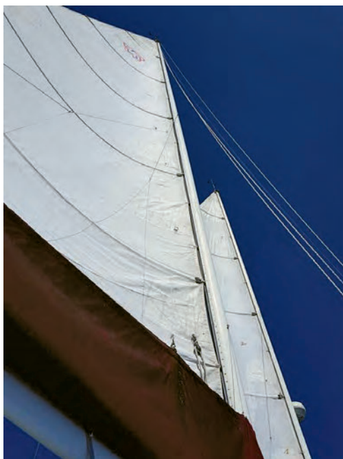
Goodwind, a 1984 Freedom 39 Pilothouse Schooner, features the original Freedom Cat Ketch rig as it evolved with full length battens and conventional booms and vang. Photo courtesy Greg Cantori.
